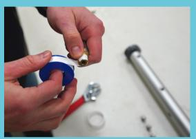
Wrap the threads of your new nozzles and filter with 4 wraps of teflon tape
