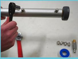
Remove original nozzles and plug - clean female threads of the chamber
