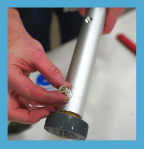
Insert the new nozzles into nozzle holes
