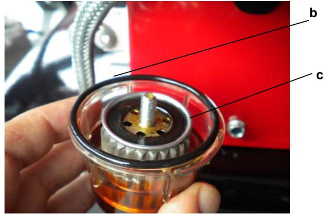
ii) Using a suitable container, collect the fuel when removing from the fuel filter assembly
